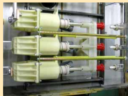
Contact system assembled in the switch
